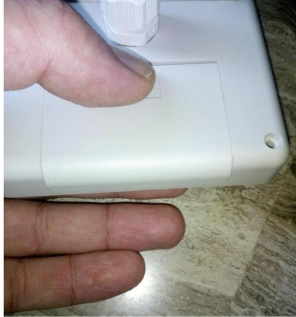
**Figure 4. Instrument's protective cap removal**
